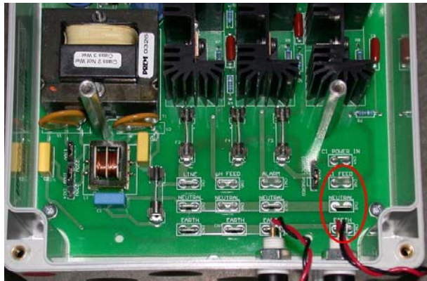
Step 14a: Wiring Relay 2 (dry contact)
